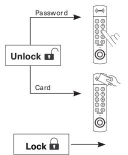
Input factory default password 1234+ ¬¬" or "4321+ ¬¬", buzzer gives out a long di... sound, the green indicator light is on, turn to unlock in 3s.
