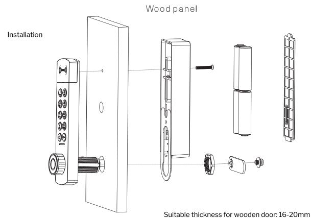
Suitable thickness for metal door: 0.6-2.0mm
